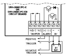
Figure 8. SRN-2000C/PC-E & -EB Wiring
