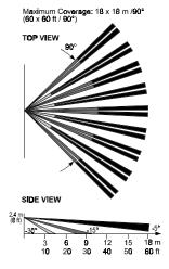
Figure 1. Coverage Pattern - Lens No. 100
