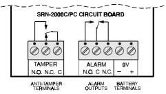
Figure 7. SRN-2000C/PC Wiring
