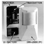
Figure 6. Back Box with Detector
