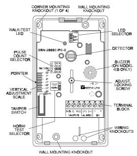
Figure 10. SRN-2000C/PC-E and -EB, Inside View
